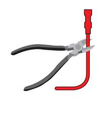
**3.** Strip back  $\frac{3}{4}$ " of the insulation with a wire stripper.
