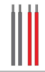
**4.** Twist both RED wires from the control board together with the RED wire from the battery harness provided. Do the same with the BLACK wires.
