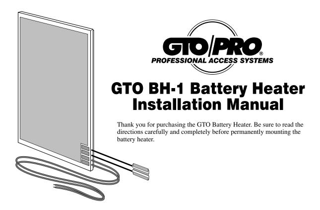
The GTO Battery heater is designed to maintain the batteries in the GTO control box at a higher temperature when the system is installed in a cold climate. The heater is easy to install and wire, and controlled by a built in thermostat that activates the heater at temperatures below 40°F (4°C). One or two heaters can be used depending on the number of batteries installed in the control box.
