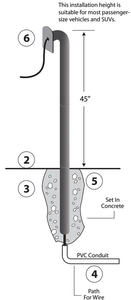
This installation height is suitable for most passenger-size vehicles and SUVs.
