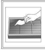
For optimal efficiency, wipe the face of the panel frequently with a soft, damp cloth.
