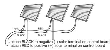
All connections should be made weatherproof using weatherproof splice kits available at hardware and electrical supply stores.
