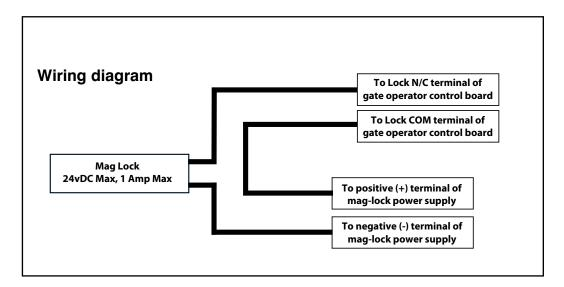
**NOTE:** GTO's GP-Series (SL050, SL100, SW050 and SW100) operators are Magnetic Lock ready with a NORMALLY CLOSED contact Lock Terminal. GTO's low voltage (2000XL, 3000XL, 4000XL, SL1000 and SL2000) operators do not have a NORMALLY CLOSED contact Lock Terminal and will require the addition of a NORMALLY CLOSED contact relay.
