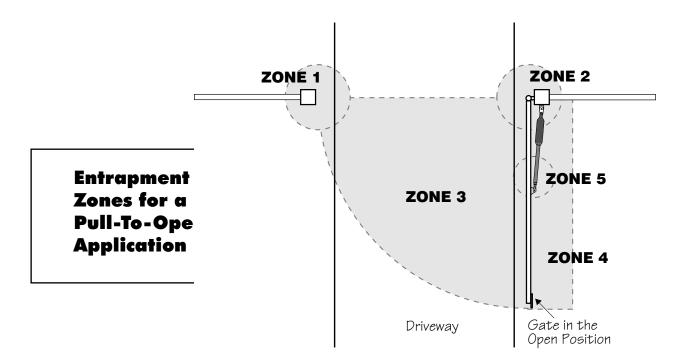
Entrapment Zones for a proper Pull-To-Open installation:
