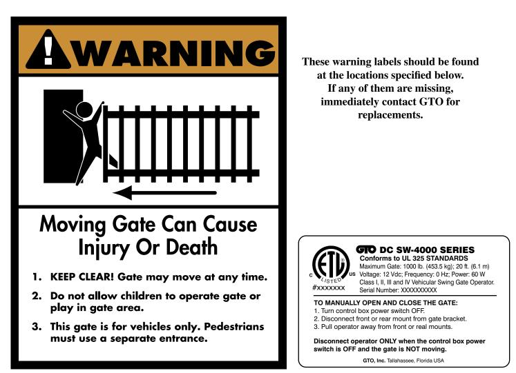
Warning signs (2 enclosed) to be installed on each side of the gate (3-5 feet above the bottom of the gate).
