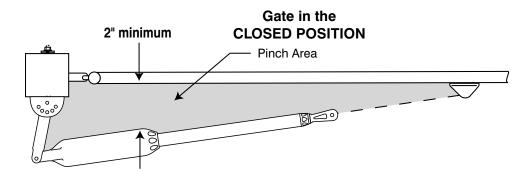
If you don't have 2 inches of clearance or the gate operator is binding on the post pivot bracket, remove the bolt in the post bracket and readjust the pivot bracket until you can achieve the proper clearance.
