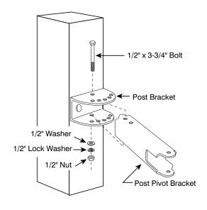
**IMPORTANT:** While determining the mounting point for the post pivot bracket assembly be sure that the position allows for maximum clearance between the gate and the operator in both the open and closed positions, as shown in the diagrams below. This clearance will give the operator the most efficient leverage point for opening and closing the gate and more importantly provides the least possible pinch area.
