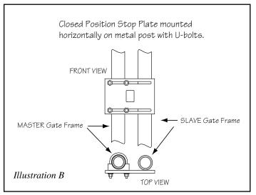
**NOTE:** The optional ground stop post is used to provide a secure point for the SLAVE gate to close against. If you will be using the GTO/PRO Horizontal Gate Lock accessory with your gate operator system, the closed position ground stop is REQUIRED, as shown in Steps 2 and 3 on the next page.
