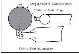
On round posts of 6" diameter or larger, the post pivot bracket may not be necessary for the installation. In this instance, the two post brackets are mounted by themselves.
