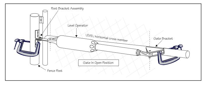
**IMPORTANT**: While determining the mounting point for the post pivot bracket assembly, be sure that the position allows for minimum 2 inches of clearance between the gate and the operator in both the open and closed positions, as shown in the diagrams below. This clearance will give the operator the most efficient leverage point for opening and closing the gate and more importantly provides the least possible pinch area.
